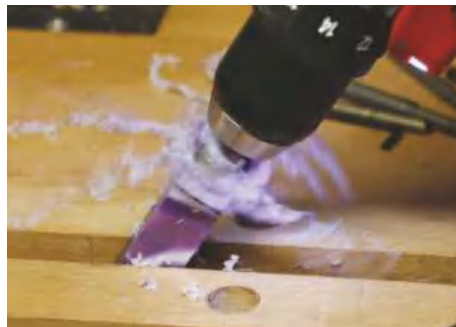
▲ Pic.3 Ream the blank back to the brass barrels ensuring you don't go too far
